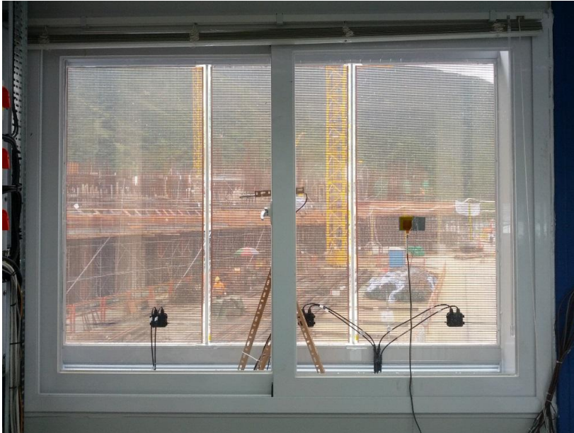
Ventilated PV window
